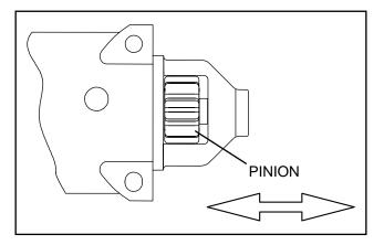
Figure 12. Check Pinion Gear Operation (V-Twin)
